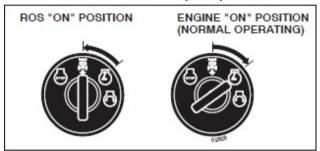
When the engine is running with the ignition switch in the engine "ON" position and the attachment clutch (PTO) engaged, any attempt by the operator to shift into reverse should shut off the engine.
